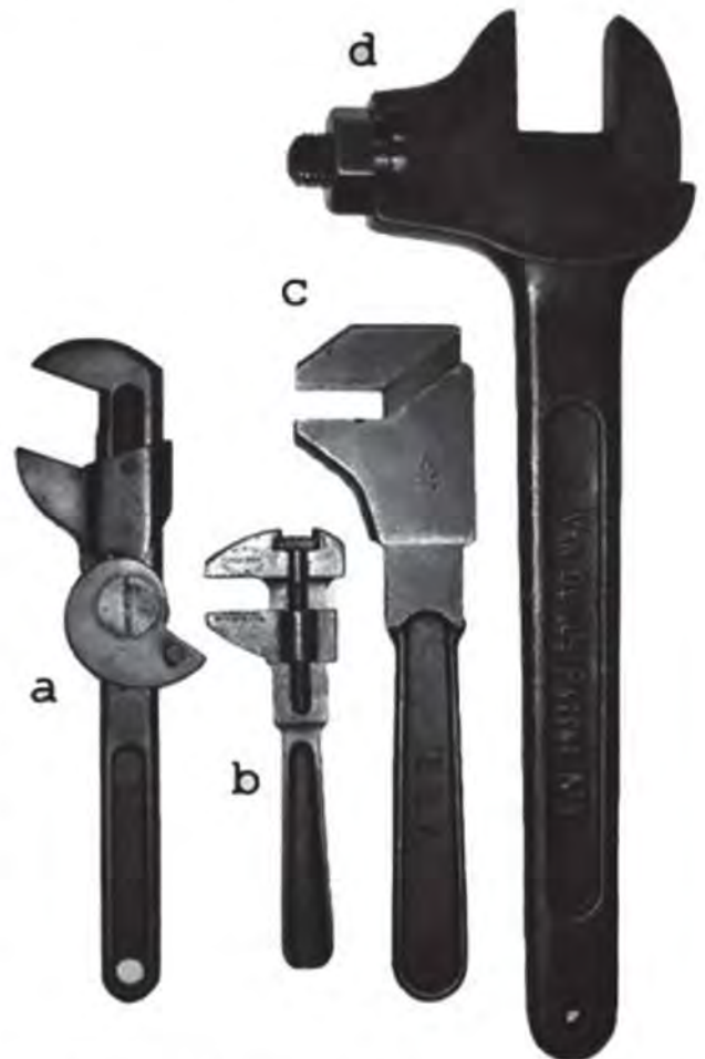
Fig. 19. (a) 9" 'Burston' eccentric cam adjuster, (b) 6" Wynn & Timmins cycle adjustable, (c) 9" BSA No. 3 'quick adjust', (d) 14½" No. 3, "van Duijl" Patent, made by Thomas Chatwin.
