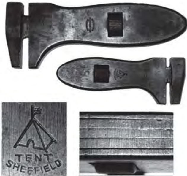
Fig. 18. Richards Bros 'TENT' brand adjustable; 6" adjustable, 4½" adjustable, riveted plates and 'TENT' logo
