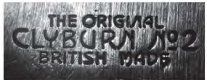
Fig. 10. The 'ORIGINAL CLYBURN' marking on a 6" Clyburn manufactured by Samuel Buckley & Co. Ltd
