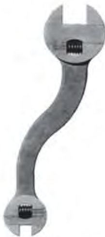
Fig. 8. Original drawing of Richard Clyburn's elongated 'S' shaped handle spanner
