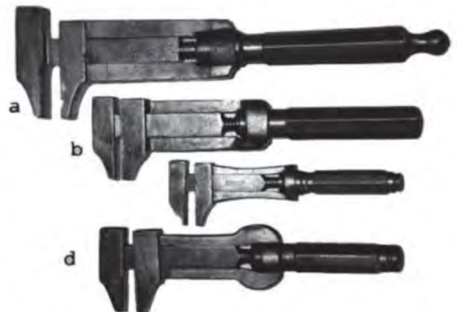
Fig. 5. French Pattern Coach Wrenches; (a) 20" I. Sorby, (b) 12 1/2" Crampton, Sheffield (c) 11" Thom Ibbotson, (d) 14" Palmer & Sons
