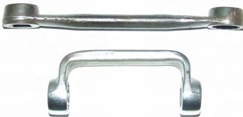
Fig. 16 - Mystery spanner beside a completed crowfoot spanner
