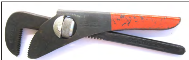
Fig. 9. Thumbturn Footprint with knurled nut and saddle adjustment.
