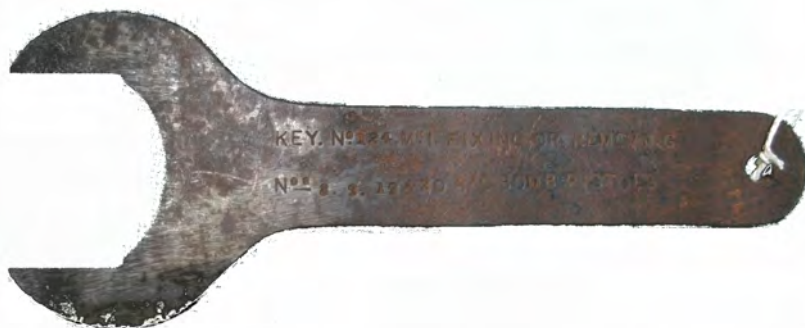
Fig. 17 - "KEY No 124 Mk 1 FIXING OR REMOVING A/C Nos 8, 9, 19 & 20 BOMB PISTOLS" other side - "PM TD -20 . 10 . 41"
