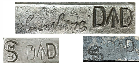
Fig 3a,3b & 3c - above McKay Massey Harris' auto or F type, profile (9in). Impressions on the upper jaw: 'Sunshine' Figurative Mark (centre), Tall S' Figurative Mark (bottom left), 'Squat S' Figurative Mark (bottom right).
