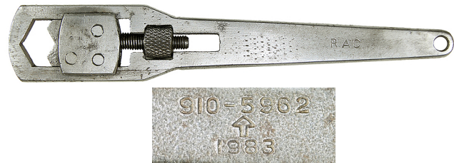
Fig 7 - The RAC captured nut, closed adjustable box type spanner, profile (7in).
