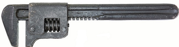
Fig 5 - Department of Defence's front rack and worm auto or F type, profile (9 ¼ in).
