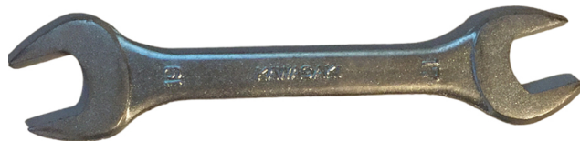
Fig 5 - Examples of Upper case letter "KAWASAKI" with DROP FORGED STEEL on reverse
