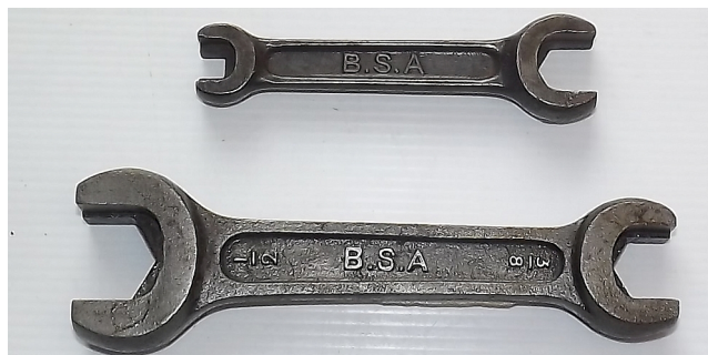
Above - comparison of the common BSA block spanner top (4"), with the very uncommon larger block spanner at bottom (6")
