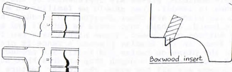
To cope with the demands of different types of wood, most moulding planes were produced in up to four blade angles. Planes intended for soft woods had their blades set at 45 degrees; this was known as the common pitch and is most
