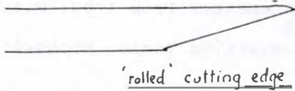
When the top is flat, the profile can be restored. I use small grinding wheels and shapes, and dunk in water often. Check the shape against the sole of the plane; it should protrude evenly at all points when the blade is in its normal position, held by the wedge. The final sharpening and honing requires a selection of small slip stones. I use oil on mine, but I don't think it matters whether you use oil or water.
